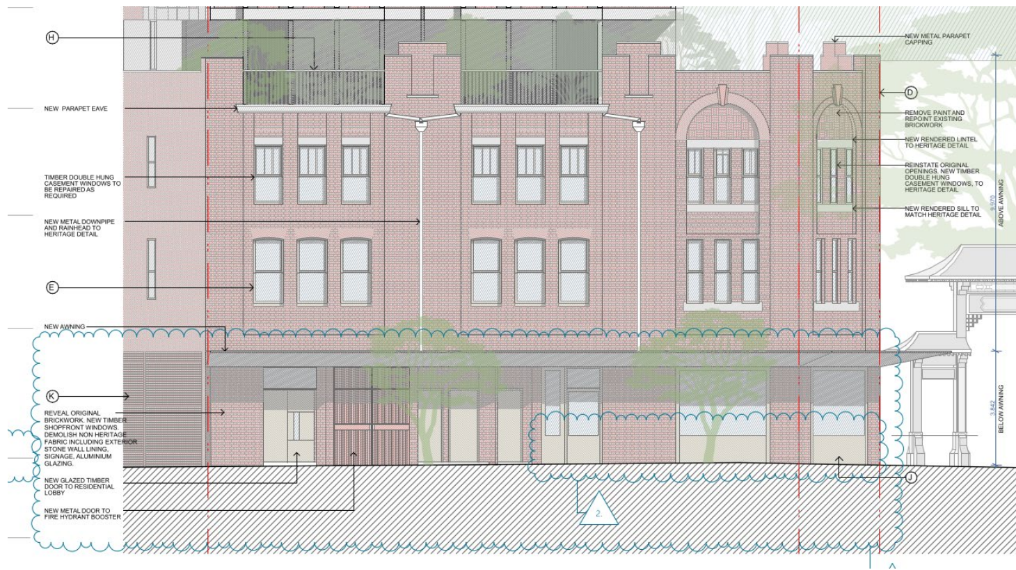
Hay Street - podium conservation works
